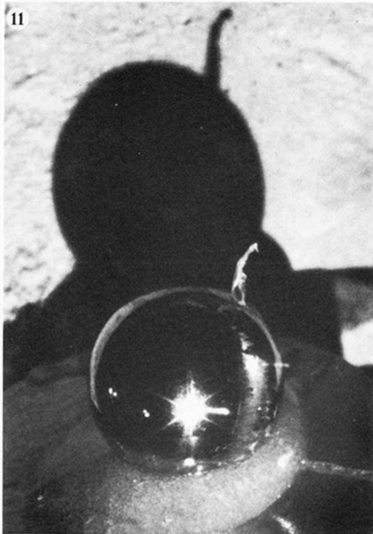
FIGURE 11. Optical picture of a filament that remained attached to a sphere after impact (ball diameter 5 mm). A shadow of the ball and filament appears in the background. v_i = 170 \pm 15 \text{ m s}^{-1} , \alpha = 36^\circ \pm 4^\circ ; v_r = 64 \text{ m s}^{-1} , \beta = 40^\circ .
